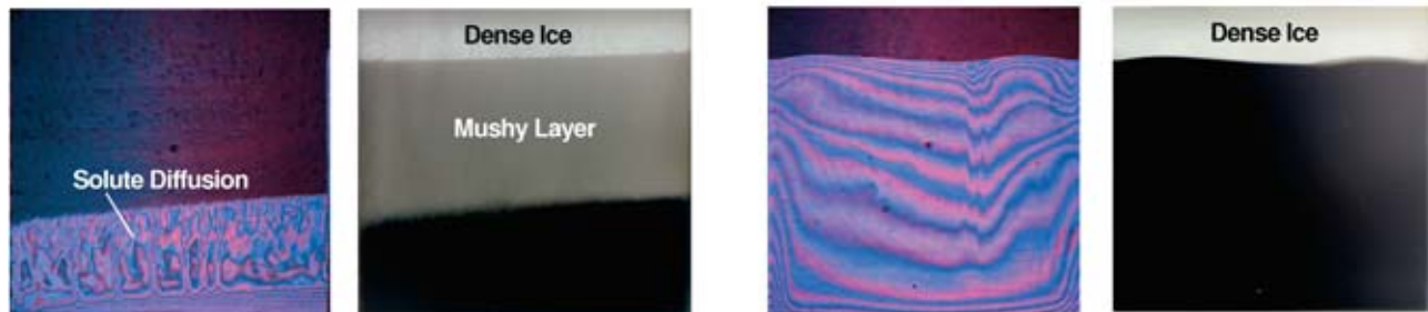
Hypo-eutectic Aqueous Solution, C_i=5\text{wt}\%
