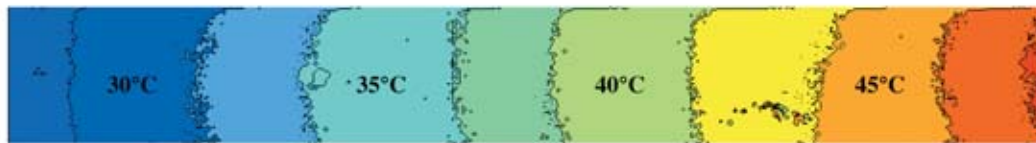
(d) Contour plot of processed temperature field showing 2.5°C isotherms
