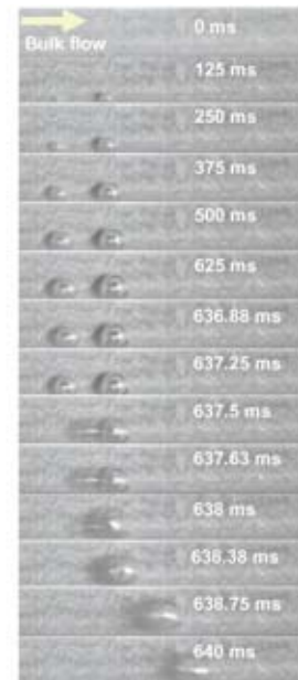
Twin bubbles agglomerate after growth and travel down the channel (8000 fps).
